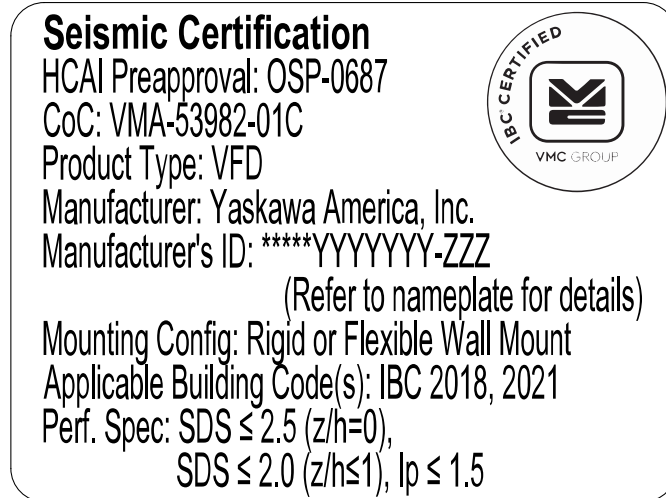
Figure 5.33 Seismic Certification Label Example for Drives
