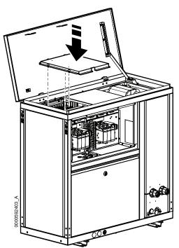
10. Close the panel and fix again the two M5x12  $\text{PHIL}^{\textcircled{\text{B}}}$  screw.
