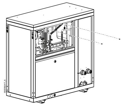
4. Open the roof panel, then lock the position by the support arm on the right side.
