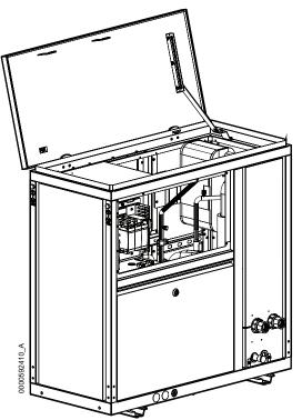
5. Remove the electrical box top panel.
