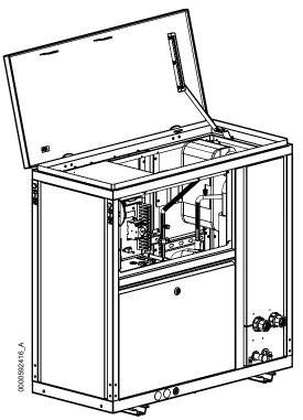
5. Remove the electrical box top panel.
