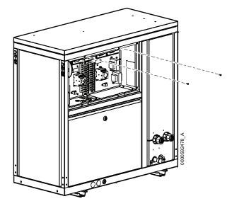
11. Install the enclosed switch shaft as shown in the pictures below.
