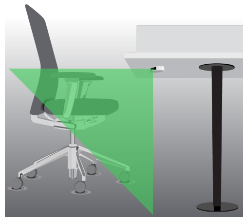
Desk Occupancy Sensor installed underneath a work desk
