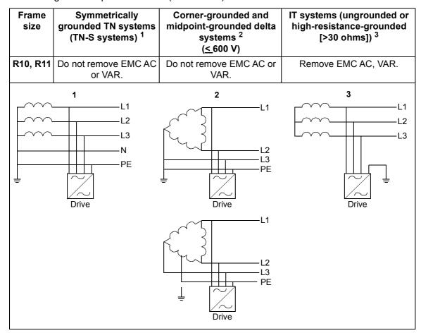
Note: These are the EMC filter and varistor screws of different drive frame sizes.
