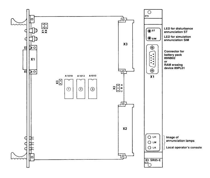
Positions of jumpers (as-delivered condition) and memory modules as well as the module's front panel
