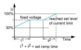
Holding the voltage at a fixed level will keep the current on the set level
