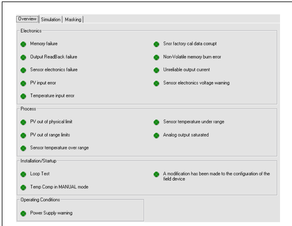
Fig. 8.2 ACA592 Toroidal Conductivity Transmitter – Diagnosis Overview Screen
