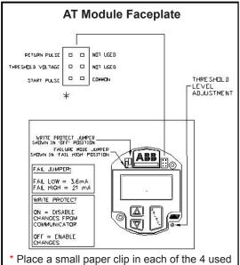
Channel A: Refer to the drawing at left for probe connections.\*
