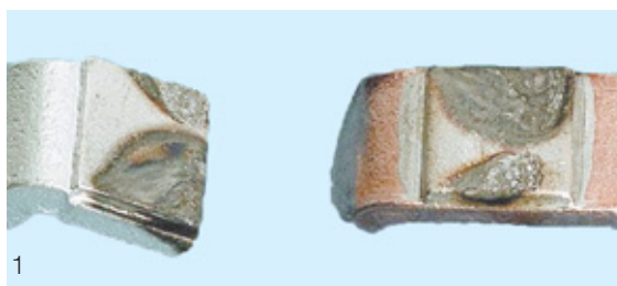
1. The appearance of contacts after a very low number of operations
