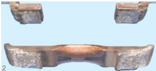
2. Mid-life stage of fixed and movable contact
