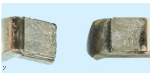
2. A contact just having reached a good worn in level
