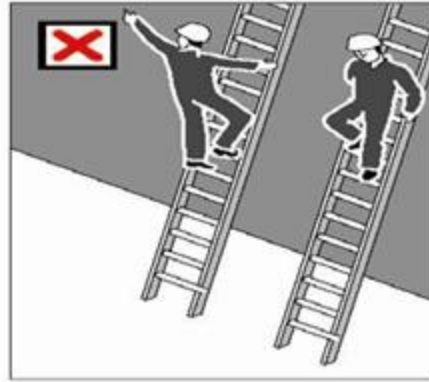
Facing away from the ladder to descend; over-reaching
