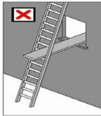
Ladder set up incorrectly
