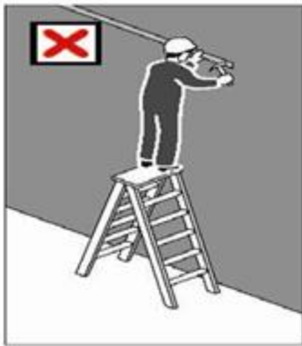
Standing on top plate of stepladder
