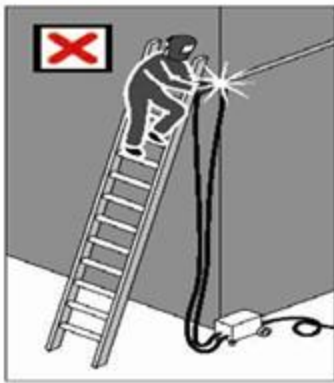
Performing hot work from ladder
