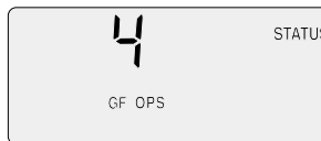
Display showing trip operations counter
