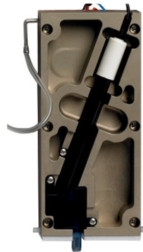
Figure 3 Electrode in temperature-controlled flow cell
