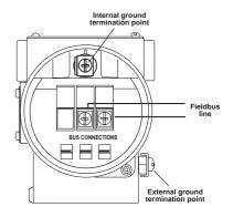
HART hand-held communicator may be connected at any wiring termination point in the loop, providing the minimum resistance is 250 ohm. If this is less than 250 ohm, additional resistance should be added to allow communications.
