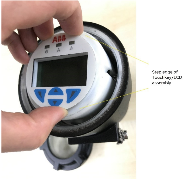
Figure 3.3: Snap the Step Edge of Touchkey/LCD Assembly
