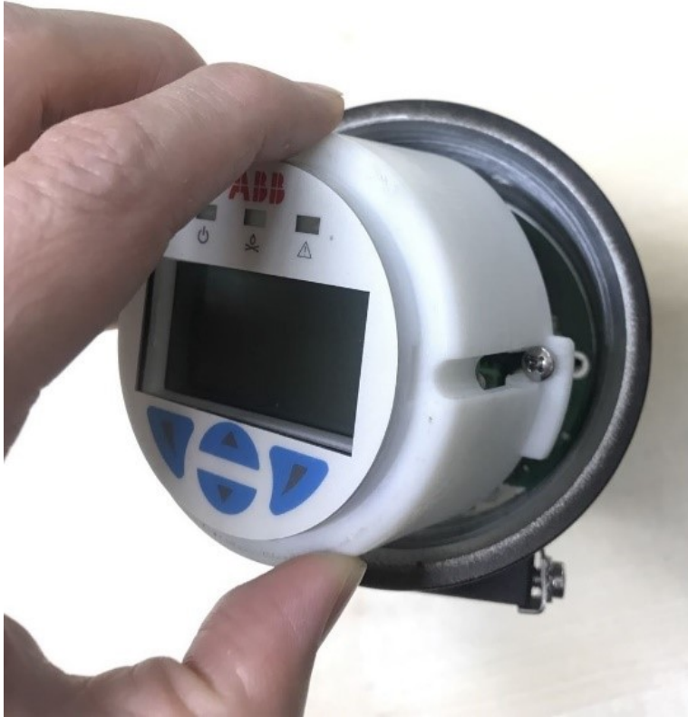
Figure 3.4: Pull and Remove the Touchkey/LCD Assembly
