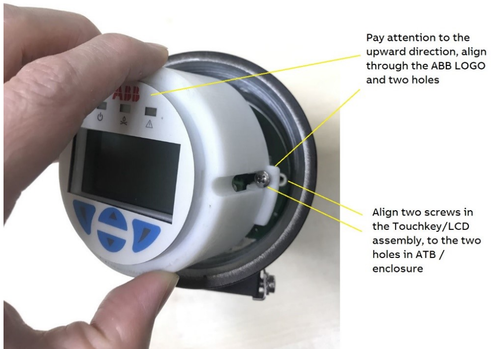
Figure 3.8: Align Two Screws in the Touchkey/LCD assembly to the Two Holes in ATB/Enclosure
