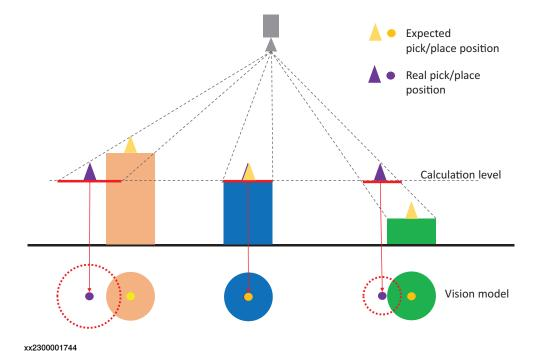
With 2.5D calibration, a full 3-dimensional space is calibrated, which allows the system to compensate for the parallax error, given that the system knows the correct height of the object. This raises the following questions:
