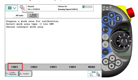
Wait for the message ...is prepared for calibration. The conveyor position in the jogging window for CNV1 should now be displayed as "0" mm.
