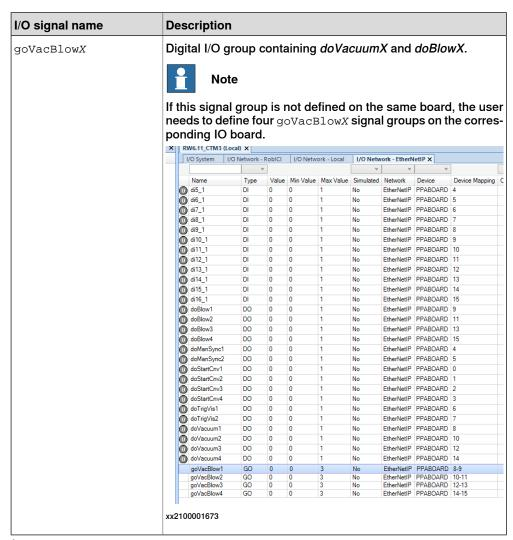
For DSQC 2000, there is no predefined port for this signal. Define the real connected port on the board as the signal name.
