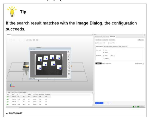
In the **Display Options** part, select **Segmentation image** to display the processed image. Select how the result will be displayed.
