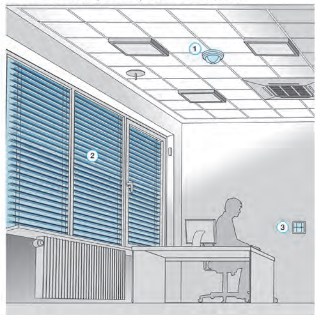
1 Presence detector | 2 Blind | 3 Manual blind control
