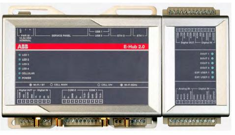
E-Hub 2.0 is an independent IoT gateway that gathers data from recognized field devices as well as pulse outputs (water/gas meters) and then connects with ABB Ability<sup>TM</sup> Electrical Distribution Control System (EDCS) cloud platform via Ethernet, Wi-Fi or cellular connectivity (GSM) for energy monitoring and measurement.
